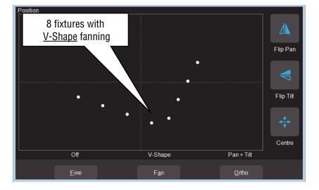
The fixture selection order is used by the Fan App. Experiment with different orders of selection to get different shapes. Previous selections can be re-used by tapping the  $\bigoplus$  [Select] button.
