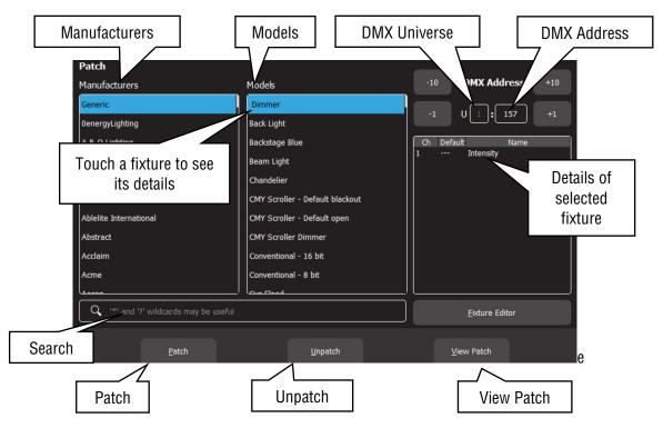
Select the fixture Manufacturer and Model of the fixture to be patched from the lists. Swipe the screen to scroll the list. Dimmers and many LED fixtures can be found in the "Generic" manufacturers listing.
